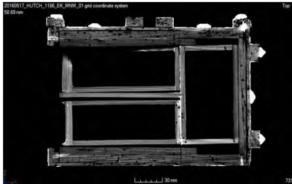
Figure 17 CT image which make visible the adhesive of the “secret” drawer.
