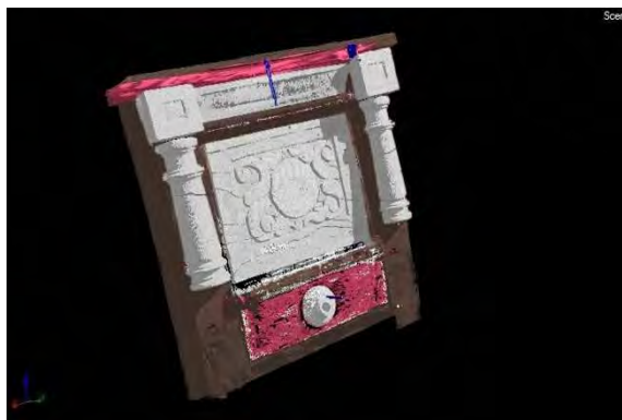
Figure 13 The different materials of the side partition: metallic nails (blue), alabaster (white), oil paint (pink) and wood (brown).
