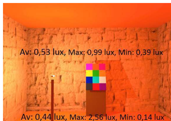
Figure 4 Photometric results for illuminance values for room with plain mud brick walls.
